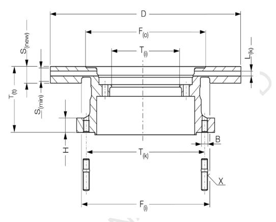
B Diameter of mounting bolt holes (or thread size in case of threaded holes)
